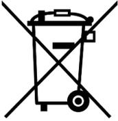
The crossed out wheeled bin symbol indicates the electric and electronic products bearing the symbol must be disposed of separate from household waste. They must be properly disposed of as waste electrical and electronic equipment.
