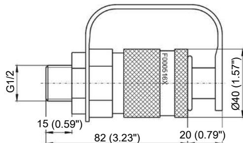
**Connection F - Filling Control Or Sealing Plug**
