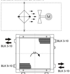
Direction of flow BLK 3-10 top left to bottom right or the exact opposite. The oil outlet is always on the opposite side. The second connection must be closed.
