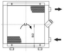
The oil inlet and outlet are always on the same side. Connections on the opposite side must be closed.
