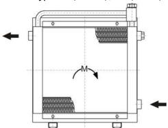
Oil inlet always at the bottom. Other connections must be closed. Oil outlet always on the opposite side.
