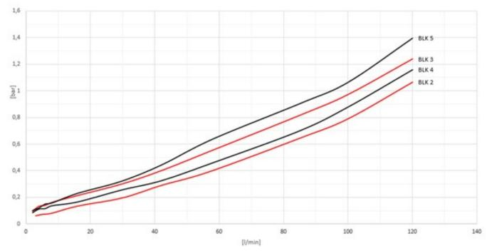
Fig. 1: Pressure loss curves BLK 2 to 5
