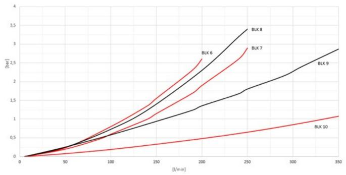
Fig. 2: Pressure loss curves BLK 6 to 10
