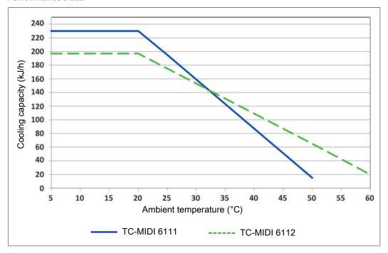
Note: The limit curves for the heat exchangers exchanger apply to a dew point of 50 °C.
