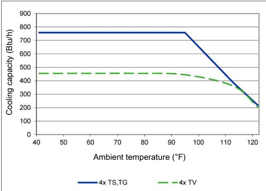
Note: The limit curves for the heat exchangers exchanger apply to a dew point of 149 °F.
