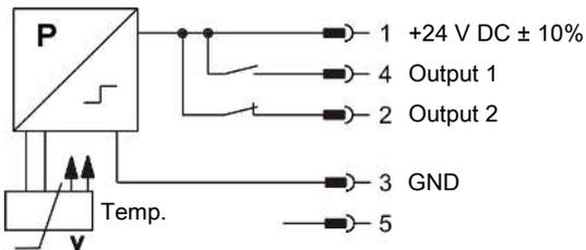
Output 1 = Alert at 2.2 bar (NO contact with rising pressure)
