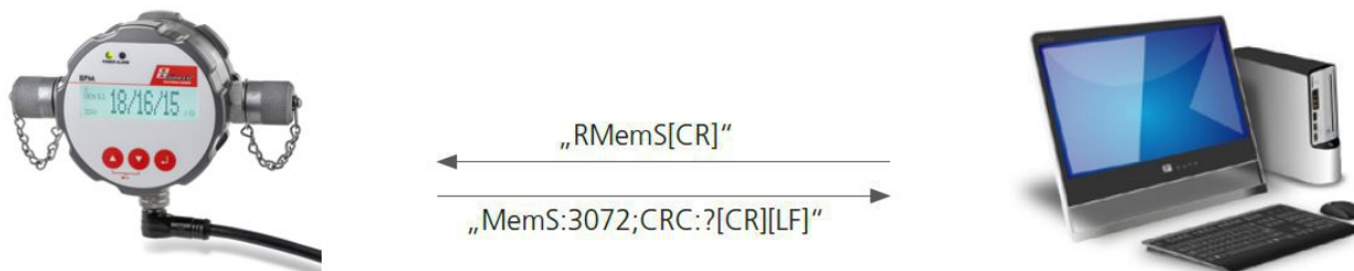
Fig. 21: Example RS 232 data transmission with checksum
