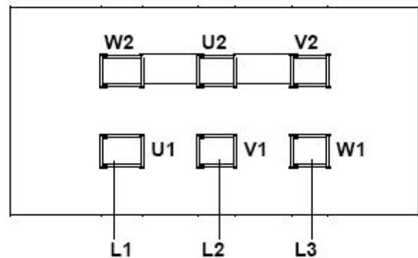
The direction of rotation can be changed by reversing any two phases.
