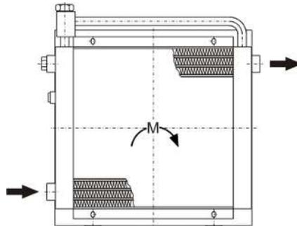
The oil inlet is always at the bottom left of the cooling battery. The second connection must be closed. The oil outlet is always on the opposite side.
