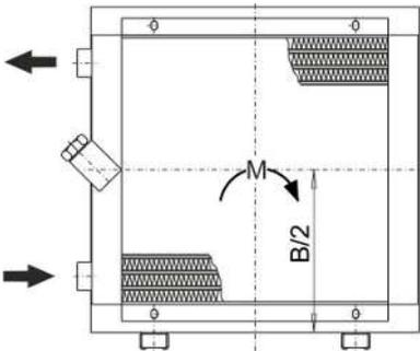
The oil inlet and outlet is always on the same side of the cooling battery. The connection on the opposite side must be closed.
