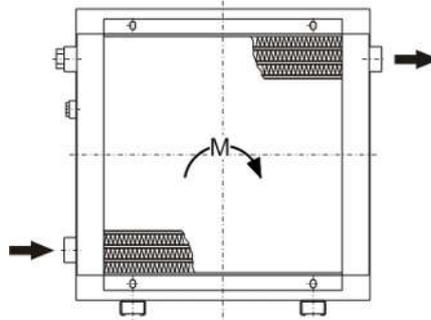
The oil inlet is on the bottom left of the cooling battery. The second connection at the top must be closed. The oil outlet is always on the opposite side.
