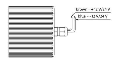
Fig. 2: Electrical connection P1.3 pumps
