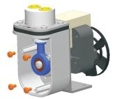
Loosen and remove the 4 Torx screws (M4x6) on the console (Torx T20).
