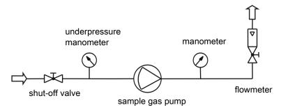
Fig. 1: Sample flow diagram of suitable monitoring
