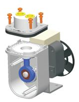
First detach the screw-in connections as described in chapter "Conversion to pump body pointing down". Loosen the 4 Torx screws M4x18 (Tx20) and lift the pump head along with mounting ring and foam cover off the console.
