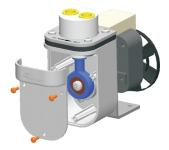
Loosen the 3 Torx screws (M3x8) on the front cover (Torx T10). Remove the cover.
