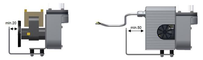
When installing the sample gas pump, always ensure an adequate amount of space between the motor and the back wall (20 mm).
