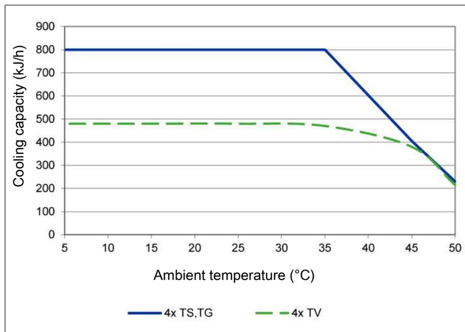
Note: The limit curves for the heat exchangers exchanger apply to a dew point of 65 °C.
