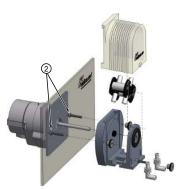
Attach the pump head bracket (3) to the gear axle.
