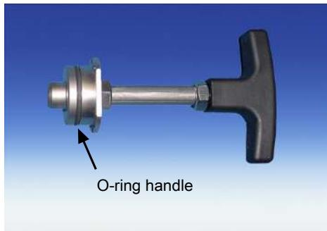
Attach an O-ring suitable for the expected ambient temperature to the handle. Attach the outlet filter to the handle. Then carefully insert the handle with filter in the gas probe and turn 90° to secure. Verify the handle is seated correctly. When seated correctly it locks onto the filter housing.
