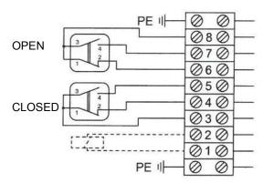
The connection diagram shows the limit switch box in the intermediate position. Switches not actuated.
