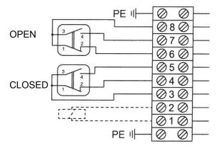
The connection diagram shows the limit switch box in the intermediate position. Switches not actuated.
