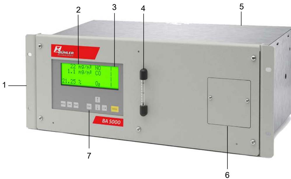
Fig. 2: Design of the BA 5000 as 19" rack unit
