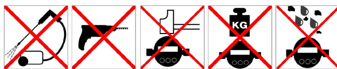
Fig. 4: Prohibited mechanical stress
