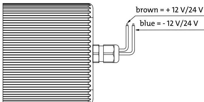
Fig. 2: Electrical connection P1.3 pumps
