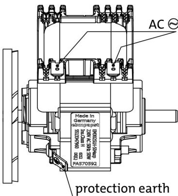
Select mains and protection earth cross section according to the rated current.
