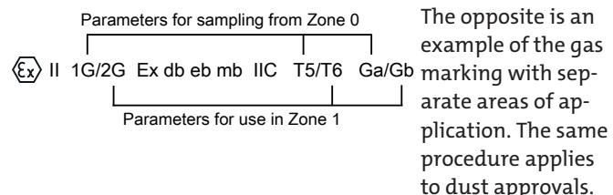
The opposite is an example of the gas marking with separate areas of application. The same procedure applies to dust approvals.
