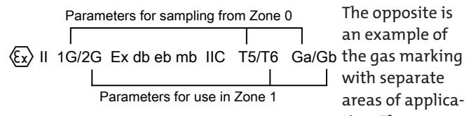
Please note, unlike the operating zone, the temperature class for sampling zone 0 is lower. This is also indicated by the ignition protection marking in the type plate.
