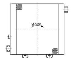
The oil inlet is on the left of the cooling matrix. The oil outlet is always on the opposite side.
