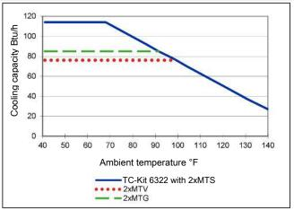
Note: The limit curves for the heat exchangers exchanger PTG, MTG, PTV or MTV apply to a dew point of 122 °F.
