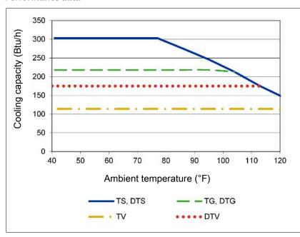
Remark: The limit curves for the heat exchangers exchanger apply to a dew point of 149 °F.
