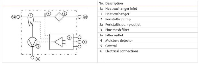
The gas to be conditioned is fed directly into the inlet of the heat exchanger (1, 1a). A hose is pre-installed between the heat exchanger outlet and the fine mesh filter (3). Sample gas is continued directly from the outlet of this filter via hose fitting (3a).
