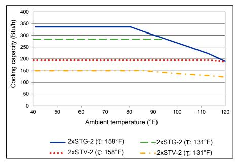
Note: The limit curves of the heat exchangers apply to different dew points (T), see legend.
