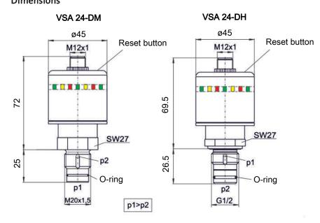
The reset button must be pressed after every filter change.
