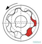
When we designed the BFP series we specifically selected the number of teeth and the width of the gerotors so the pumps have the smallest possible physical dimensions, low weight and minimal loss in efficiency. The low relative speed between the internal and external gear make the pumps extremely durable and smooth.
