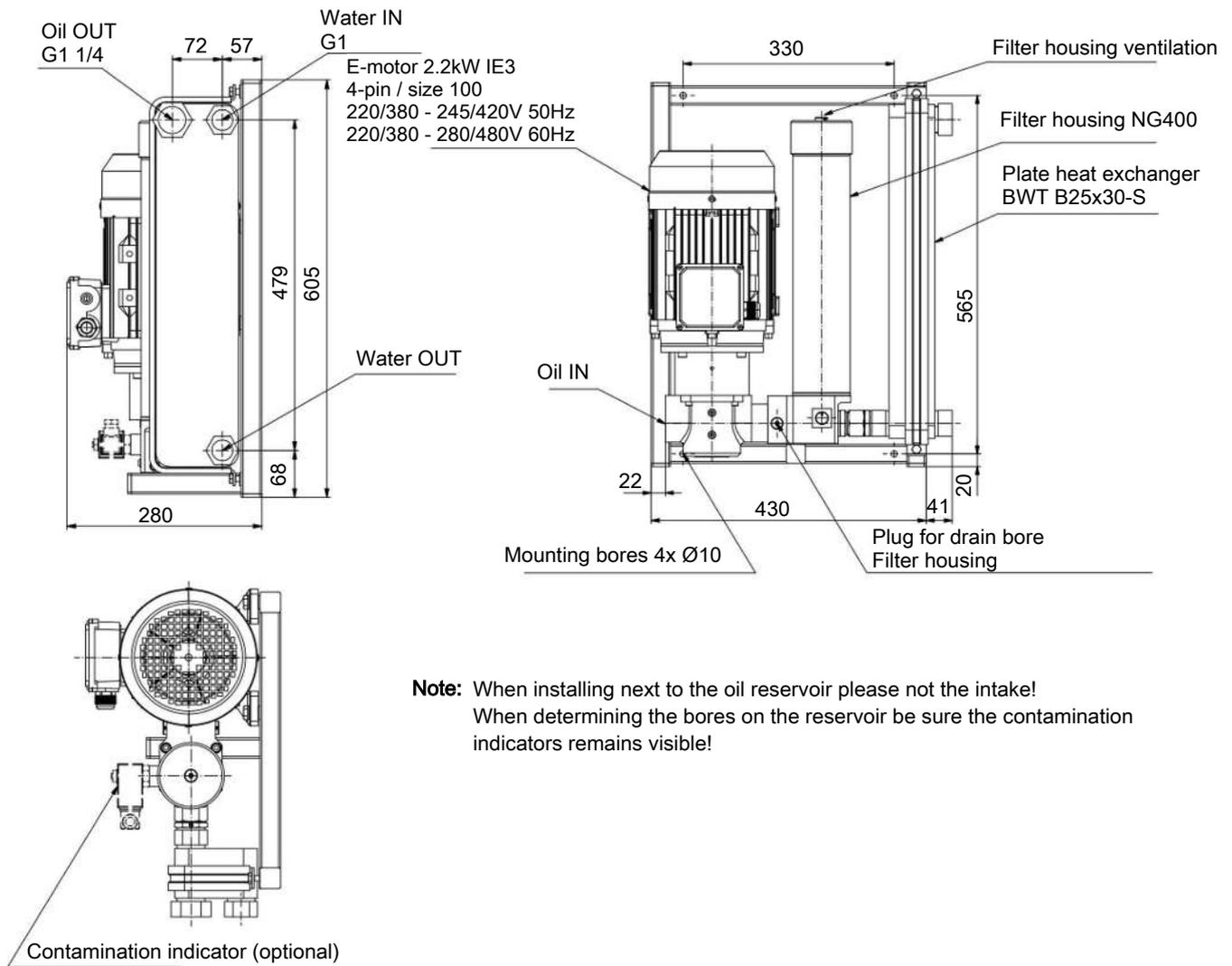
**Note:** When installing next to the oil reservoir please not the intake!
