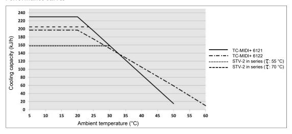
Note: The capacity of STG-2 heat exchanges is equivalent to the maximum cooling capacity of the cooler.
