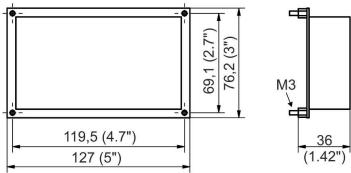
Power board (option expansion module 24 V)
