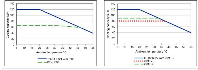
Note: The limit curves for the heat exchangers exchanger PTG, MTG, PTV or MTV apply to a dew point of 50 °C.
