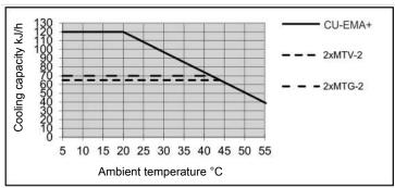
Remark: The limit curves for the heat exchangers MTV-2 and MTG-2 apply at a dew point of 50 °C. Depending on the installation version, the cooling capacity curve may vary.
