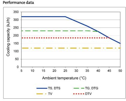
Remark: The limit curves for the heat exchangers exchanger apply to a dew point of 65  $^\circ C.$
