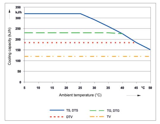
Remark: The limit curves for the heat exchangers exchanger apply to a dew point of 65  $^{\circ}$ C.
