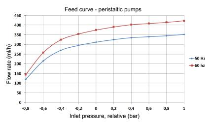
When operating the pumps with 60 Hz, the values increase by 20 %.
