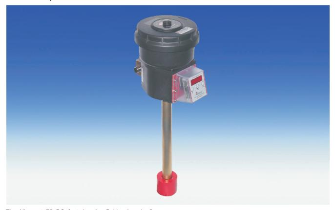
The Nivovent 75 DC featuring the Buhler "easyjust" technology is a compact economic combination of level switch and precise temperature control with LED display. The unit can provide two temperature alarm/switch outputs in addition to two level contacts.
