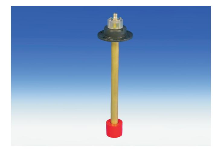
By researching existing standards for fluid power packs including DIN 24346 regarding liquid level control, it was found that measuring to 11.8" depth was sufficient to control the level. Therefore the Buhler standard length of 14.6" is sufficient and covers most applications. Flange mounting is almost universal for breather/filler units so it is also suitable for mounting level controls.
