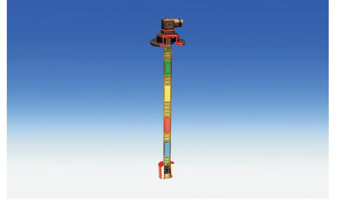
The new Buhler "easyjust" system simplifies the adjustment of level contacts. The system consists of level contact cartridges that clip onto a gold plated contact board. This board can accommodate up to four contact cartridges plus the temperature control. The temperature control is a bimetal switch. Both the level contacts and the temperature control clip directly onto the contact board thus eliminating wiring.
