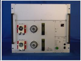
The Buhler Model SCS Sample Gas Conditioner is a pre-engineered, pre-packaged sampling system including all pneumatic components that are normally used in gas analysis systems. The SCS integrates the following pneumatic functions: sample pump, sample cooler, calibration gas valves, flow meters, condensate drains, particulate filtration, and operator interface, PLC or data logger control features all into a single 19" rackmount enclosure.
