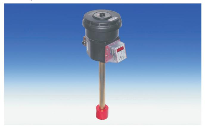
The Nivovent 75 DC featuring the Bühler "easyjust" technology is a compact economic combination of level switch and precise temperature control with LED display. The unit can provide two temperature alarm/switch outputs in addition to two level contacts.
