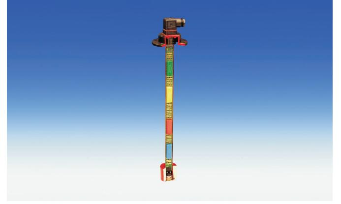
The new Bühler "easyjust" system simplifies the adjustment of level contacts. The system consists of level contact cartridges that clip onto a gold plated contact board. This board can accomodate up to four contact cartridges plus the temperature control. The temperature control is a bimetal switch. Both the level contacts and the temperature control clip directly onto the contact board thus eliminating wiring.
