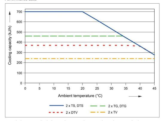
Note: The limit curves for the heat exchangers exchanger apply to a dew point of 65  $^{\circ}\text{C}.$
