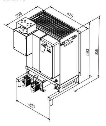
Mounting holes  $445 \times 420 \times \emptyset10$  (wide x high x diameter)
